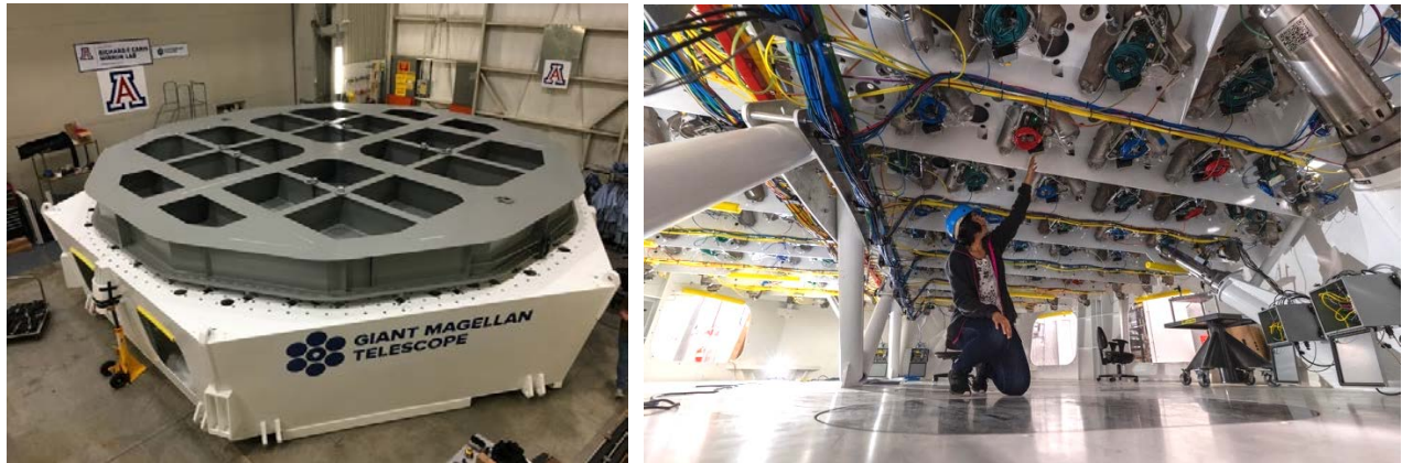
Figure 8. Test cell with steel surrogate mirror (left) and interior layout of the active optics support system (right). Work is being performed at UA. Photos courtesy of UA.
