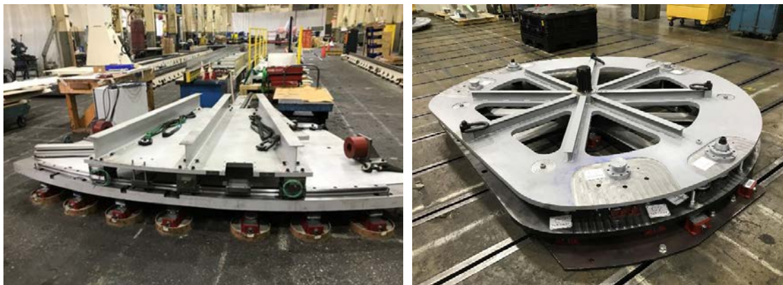
Figure 5. Prototype testing also includes a GIR bearing segment performance test (left) and sub-scale mirror cell positioner alignment and repeatability test (right).
