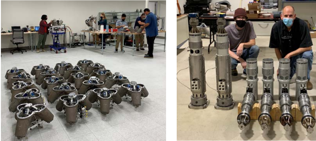
Figure 7: Triple-axis support actuators (left) and hardpoint actuators (right) being prepared for integration into the test cell.
