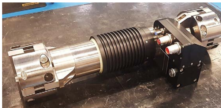
Figure 12. Prototype hexapod positioner actuator is undergoing testing at ADS.
