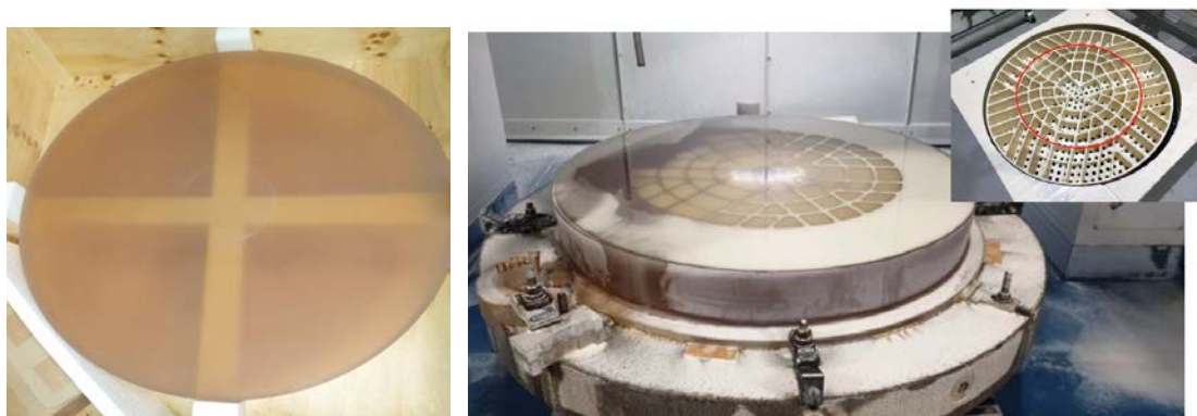
Figure 11. Zerodur blank material for the thin shell (left) and reference body (right, undergoing machining).
