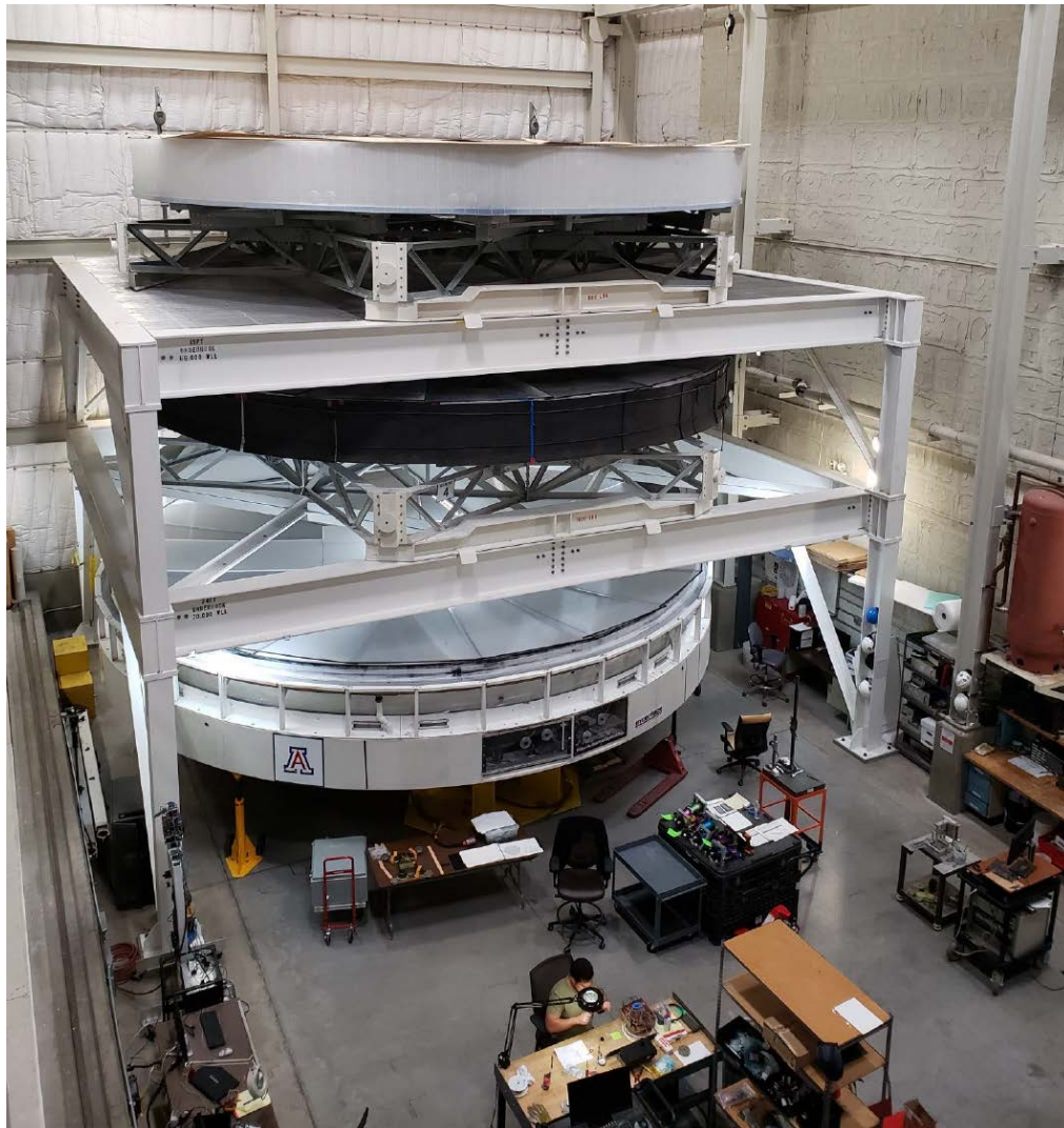
Figure 9. Primary mirror segments 4 (middle), 5 (bottom), and 6 (top) are shown in the mirror stacking rack at RFCML. Segment 5 will be the next to undergo front surface polishing, following acceptance testing of segment 3. Segment 6 is awaiting access to the grinding machine. Photo courtesy of UA.
