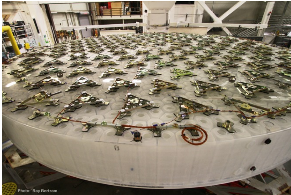
Figure 3. The second GMT off-axis mirror segment, face down, with the load spreaders for the support system attached.
