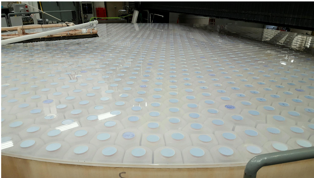
Figure 4. Primary mirror segment 3 following completion of rear surface polishing.
