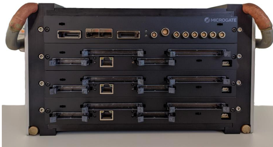
Figure 6. P72 sub-scale prototype control crate.
